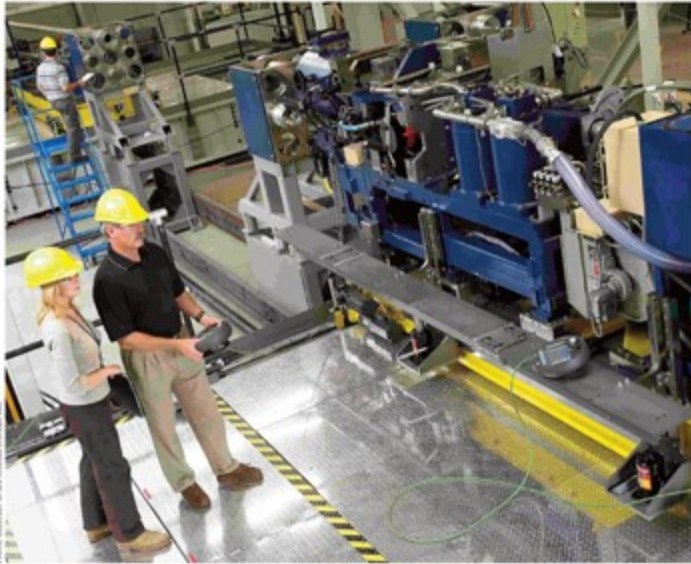
Technicians test the AECL nuclear generator refurbishment equipment in the simulation room at the ATS facility in Cambridge.
